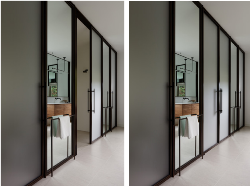
(above) After view. A simplified rhythm of bronze panels of frosted glass and mirrors unifies one wall of the bathroom to hide two toilet rooms and shower. (left photo shows opening to shower)
